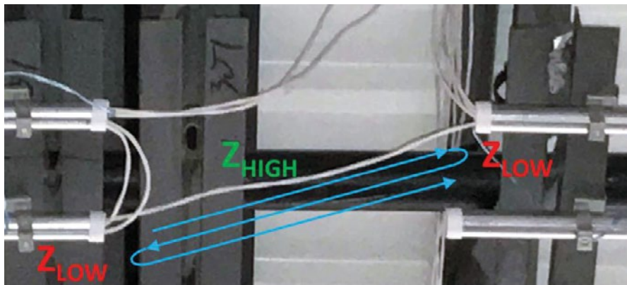
Figure 4. Impedance discontinuities creating a standing wave, example 1.
