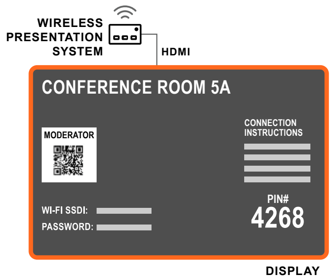
FIGURE 4: Incoming presenters are greeted with a welcome screen and instructions for sharing content to the display.
