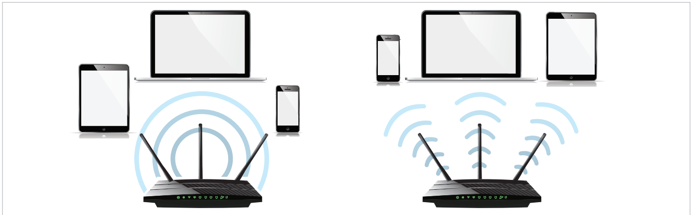
Figure 3. Example of beamforming with one spatial stream (left) and three spatial streams (right) 3 .
