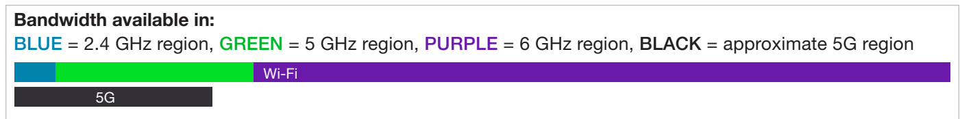
Figure 4. Comparison of available bandwidths of Wi-Fi and 5G.
