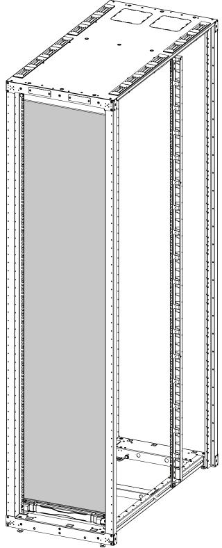
Pins of Blanking Shade must lock into Rail holes to lock Shade position.
