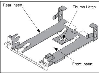
Figure 1: FLEX-OPTI-1RU removed from packaging
