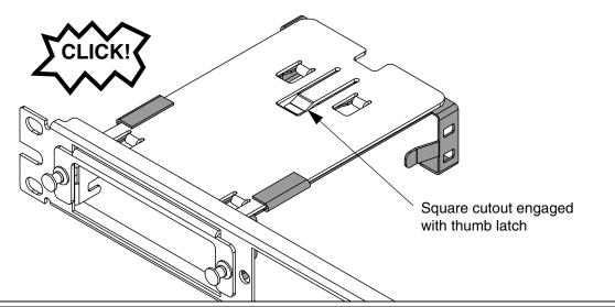
Figure 8: FLEX-OPTI-1RU rear insert square cutout engaged with front insert thumb latch, seated into final position
