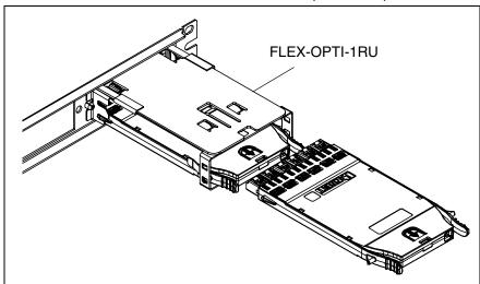
Figure 13: Upper cassette oriented to be inserted into FLEX-OPTI-1RU
