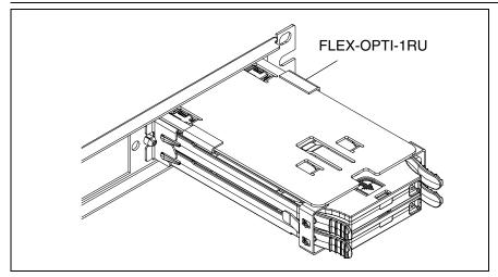
Figure 15: Upper cassette fully installed into FLEX-OPTI-1RU
