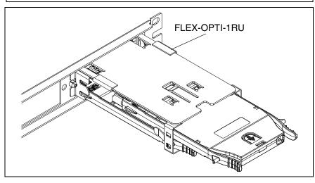
Figure 14: Upper cassette partially installed into FLEX-OPTI-1RU
