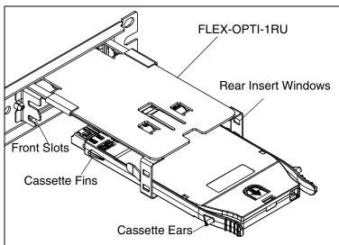
Figure 11: Lower cassette partially installed into FLEX-OPTI-1RU
