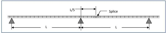
Figure 5: Splice Location in Relation to Supports, Side View
