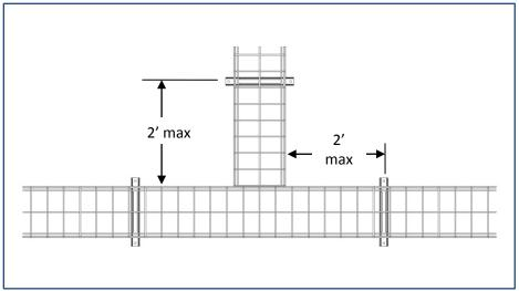
Figure 7: Support Recommendation for Horizontal Tee Intersections, Top View
