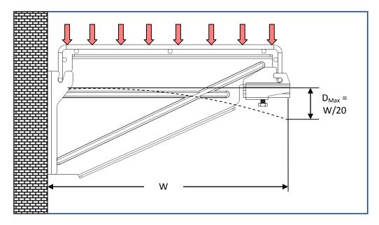
Figure 4: Cantilever Bracket Deflection
