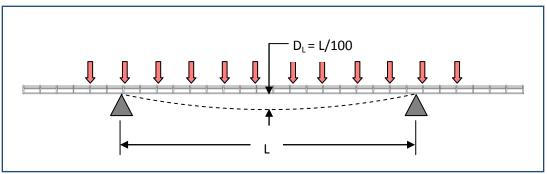
Figure 1: SWL Test Schematic, Side View
