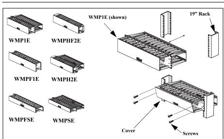
Install the managers to the rack with the #12-24x.5 screws provided. Built-in screw retention in mounting holes secures screws in manager during installation. Install the covers to the manager by positioning cover flat against the front of the manager fingers, then push to snap in place.
