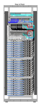
In this diagram, the Appliance Nodes are deployed from the bottom up and the switches are populated from left to right. White and black cables demonstrate the routing of SFP28 25 Gb/s Direct Attach Cable Assemblies. Aqua color cables represent the pathways of OM4 fiber uplinks. Inner switch connectivity is shown in red, while RJ45 out of band management cables are depicted in blue. Appliance connectivity shown on the left is listed below.
