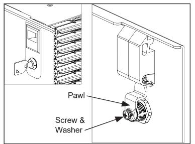
Install the pawl onto the flats of the cylinder and secure with the screw and washer.
