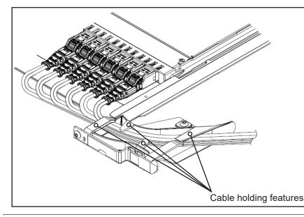
Route the cables under the cable holding features, as shown.
