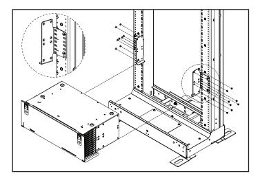
Carefully slide the enclosure onto the bottom horizontal flanges of the mounting brackets, making sure the enclosure is slid fully into place.
