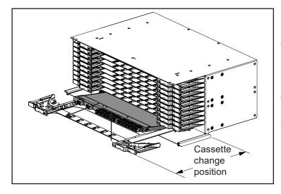
Cassettes can be installed and removed from the front of the enclosure as needed for replacement or migration. Open door and slide tray out slowly until it clicks into the second stop position, the cassette change position. Disconnect patch cords from the front of the cassette if replacing/removing cassette. Lift cassette up from the front to disengage it from the tray and remove.
