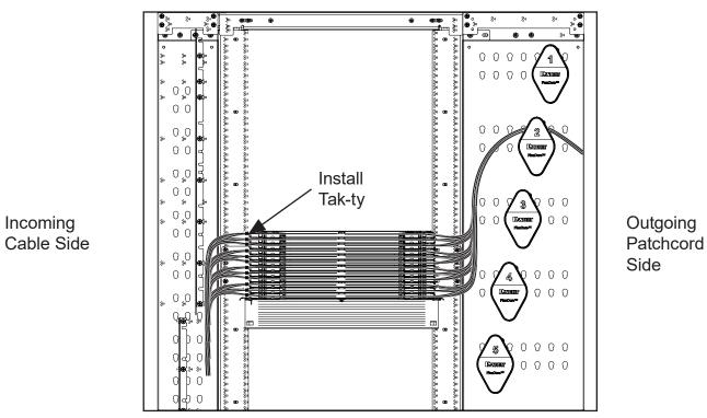
In the configuration shown above, install patch cords into the front of the cassettes working from left to right, starting with the bottom most tray. It is recommended to populate each tray across before moving to the next tray above. Route patch cord upward to corresponding spool. Repeat process until all patch cabling is installed. Route incoming cables per FS206 and patchcords per FS204.
