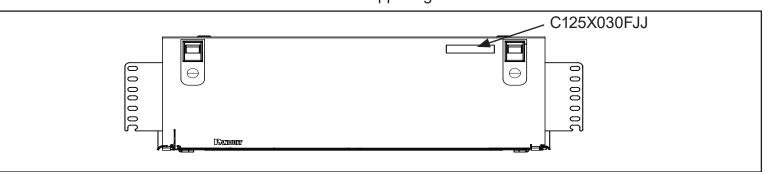
Apply the 12 sets of pre-printed part # C125X030FJJ labels provided to both sides of each tray. Cassette port numbers may be printed onto these tray labels. Tray 1 is shown below as the lowermost tray and tray 12 is on the topmost tray. Optionally, tray 1 can be the topmost tray.
