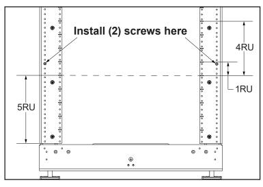
Locate two (2) #12-24 screws from FLEX-KIT to attach the enclosure mounting brackets to the Flexcore ODF rack.
