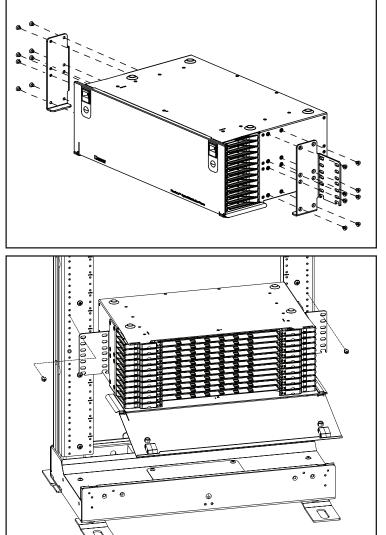
Install mounting brackets using (16)  $\#10-32 \times 1/4$  Flat head screws
