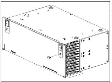
Remove the plug in the door to exposed the lock hole. The lock can be installed on either or both sides of the door.
