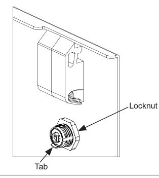
On the rear door surface, install the lock in the lock hole, with the tab of the lock body in the bottom position, as shown. Secure the lock with with the locknut.
