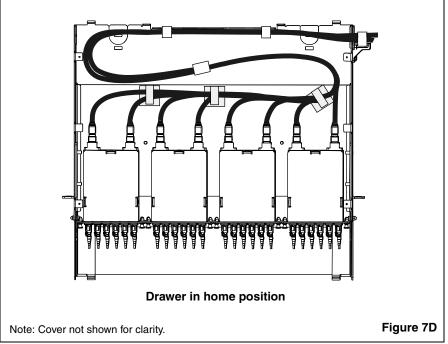
Route fiber through grommet to fiber cassettes as shown. Leave enough slack so when the drawer is fully extended the cables are not put under tension. DO NOT use so much slack that the drawer cannot be returned to its home position. (See Figure 7D)
