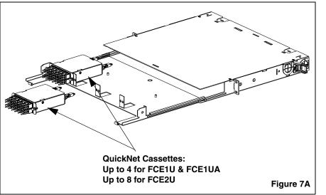
Depress spring latch and pull sliding tray out to the extended position.
