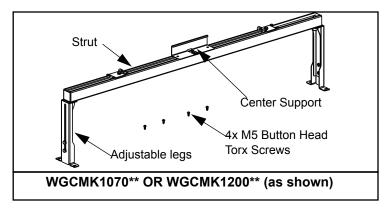
Note: The cabinet Mounting Brackets in the depicted configurations are capable of supporting Wyr-Grid Pathways at their safe working load unless otherwise noted.
