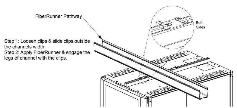
Step 3: Tighten both clips to 4 Lb-ft (5.4 N-m)
