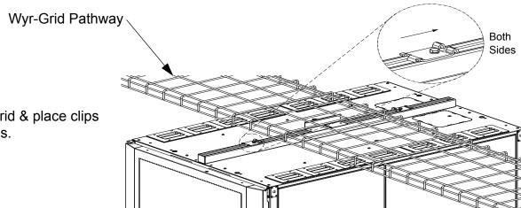
Step 1: Position Wyr-Grid & place clips over the pathways wires.
