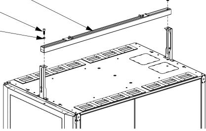
Step 3: Adjust the height of the Strut to the desired height.
