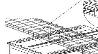
Step 2: Tighten both clips to 4 Lb-ft (5.4 N-m)
