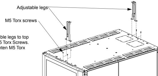
Step 1: Attach adjustable legs to top of cabinet using (2) M5 Torx Screws. (each leg) (Do not tighten M5 Torx screws)
