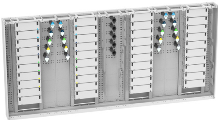
Cross Connect four frame lineup with end panels and over length storage - 300mm wide intermediate VCM (Recommended patch cord length between two double frames is 10m)
