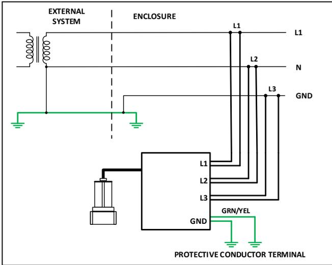
**Single-Phase: 2 Wire + PE, Redundant Detection Lead**
