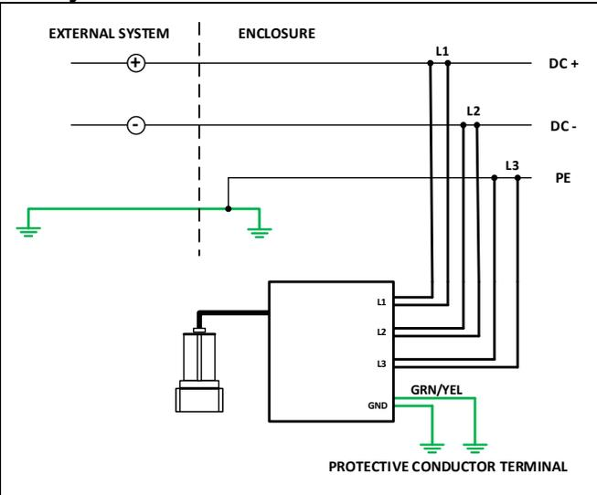
**DC System: 2 Wire + PE, Redundant Detection Lead**
