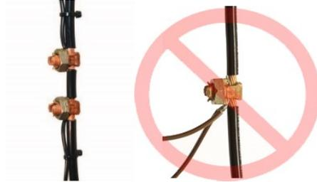
7. Terminate the sensor and ground leads. Secure the sensor leads to the conductors and insulate the connections.
