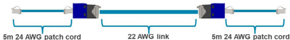
Figure 1: 22 AWG link under test with a total of 10 meters of 24 AWG patch cords
