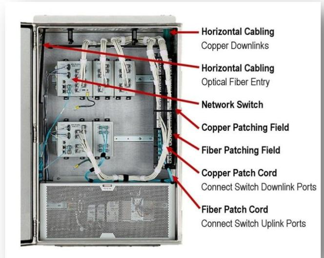
**Figure 4. Integrated Network Zone System permanent link implementation.**
