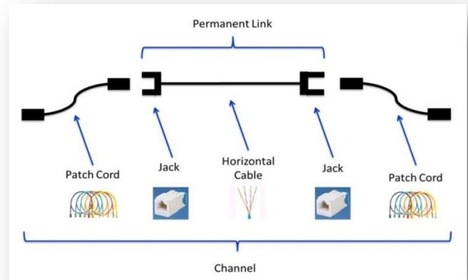
**Figure 3. Simplified Example of Copper Structured Cabling.**
