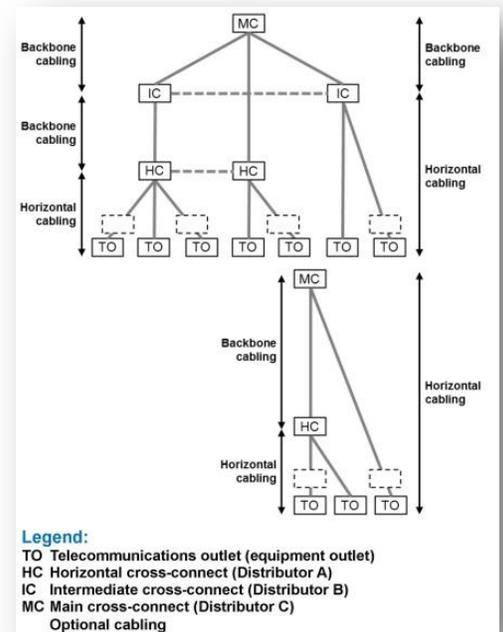
**Figure 2. Elements of a Generic Cabling Topology.**
