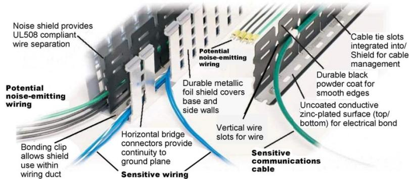
**Figure 8. Noise shielding solutions can reduce the effects of EMI/RFI (electromagnetic interference, radio frequency interference) and provide space optimization within industrial control panels.**
