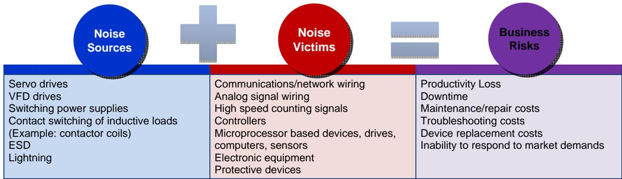
Due to the close proximity of sensitive devices to noisy sources, the leading modes of EMI within an enclosure are capacitive and inductive coupling. Understanding both sources helps to examine how best practices and specifying noise mitigating products improve equipment reliability.
