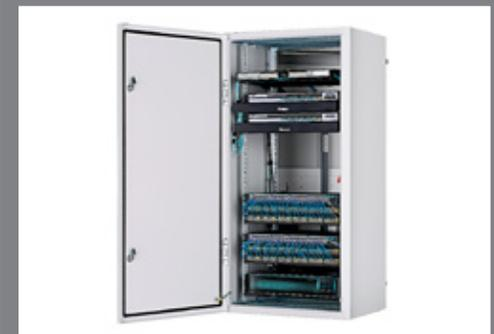
The Pre-Configured IDF is specifically engineered to deploy and protect rack mount Ethernet switches in industrial applications. Extra-depth allows room for cable management, power management, and switch stack cables and accommodates up to 5 switches. The innovative design provides consistent equipment deployment with faster installation and can significantly lower the risk of downtime due to switch overheating.
