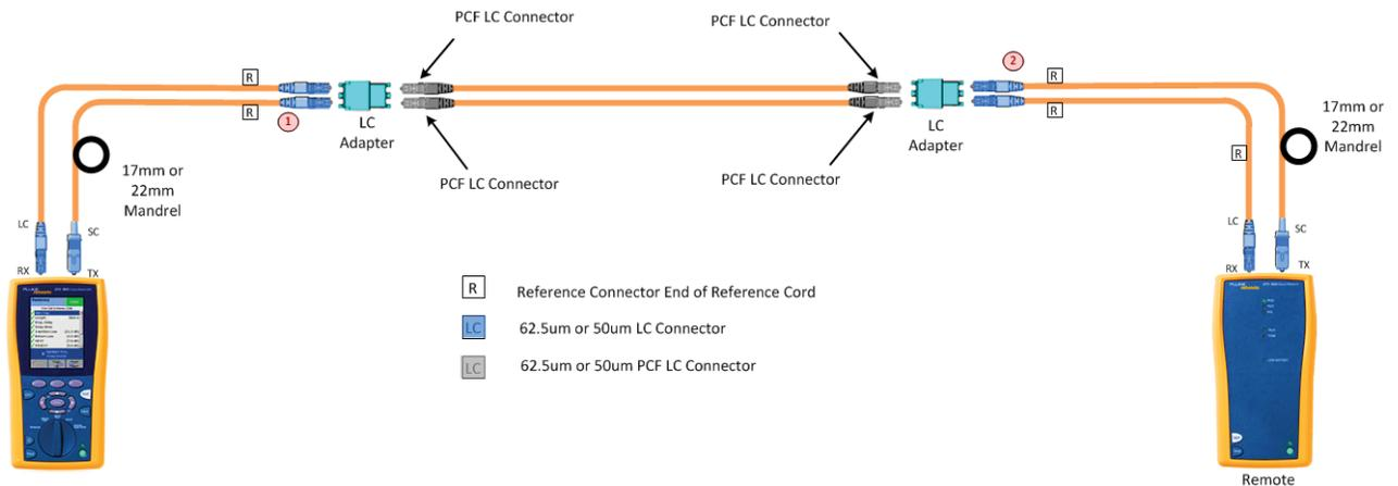
4. Connect the PCF fiber cable and connectors as shown in the figure above.
