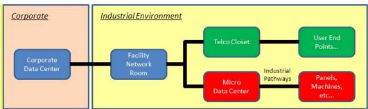
Figure 3. Block Diagram Indicating Location of Micro Data Center in Relation to the Data Center, Corp Network, Industrial Pathways, and Equipment Panels
