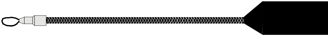
Figure 4: Completed grip setup on outside plant ribbon stranded loose tube cable using CSM and OSM only
