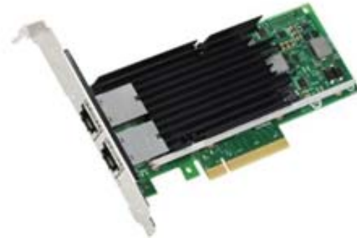
Figure 7. Intel® Ethernet Converged Network Adapter X540-T2.
