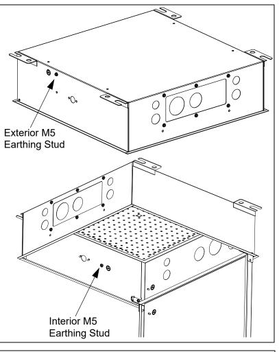
MSGK door bonding kit (sold separately) includes one quick-disconnect jumper to bond the door to the enclosure. Attach each end of the bonding jumper to the specified M5 bonding studs using the bonding nuts provided with the MSGK kit.
