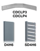
PanelMax™ Corner Wiring Duct is used in the vertical corners of medium to large electrical control panels to route, conceal, and protect electrical wiring. Reclaims up to 20% panel space by utilizing the previously unusable corner space, and improves aesthetics by providing a clean transition of wiring from the back panel to the side panels.
