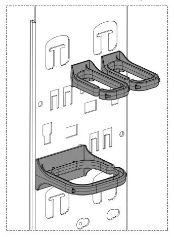
Install Flex-Clip 18 & L-Rings in orientation shown. (Reference Installation Instructions CM615C for further Information.)
