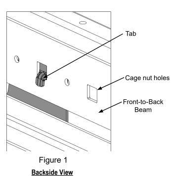
VCMP Tabs engage the cage nut holes on Front-to-Back Beam of cabinet frame
