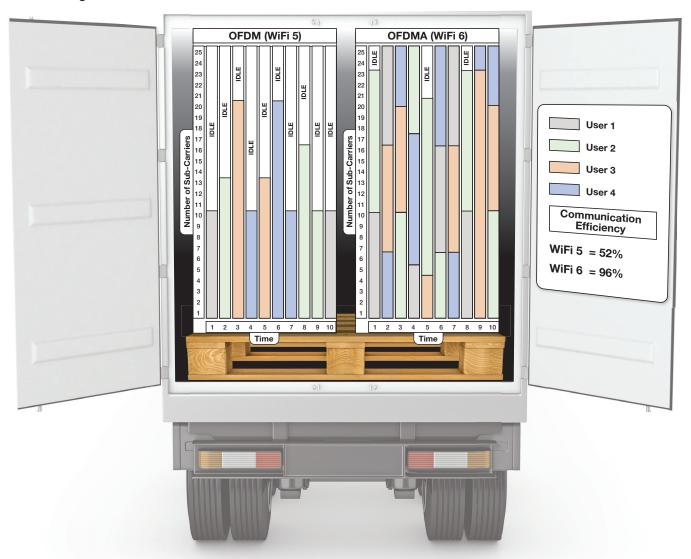
Figure 2. OFDMA in Wi-Fi 6 allows for more efficient use of bandwidth versus OFDM, as visualized by pallets in a truck. This improves throughput while reducing latency.
