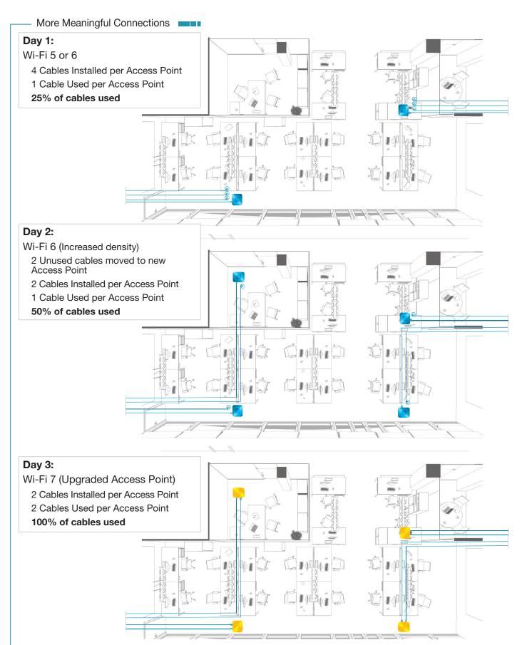
Figure 5. Example of four cables per access point being used to increase density (Day 2) and to support port aggregation for upgraded access point performance (Day 3), all using the same cabling infrastructure installed on Day 1.
