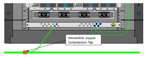
Figure 2: Cabinet Ground Jumper Going Down to Underfloor MCB
