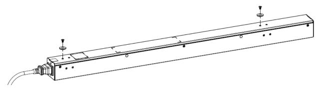
2. Install the PDU by inserting the mounting buttons into the keyhole slots on the PDU mounting bracket in the rack.
