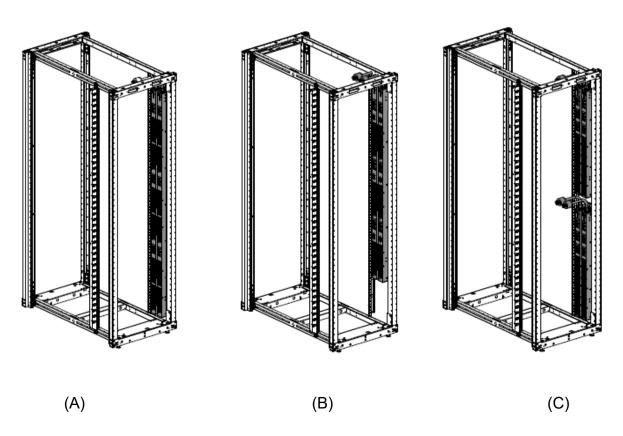
**NOTE:** (A) Two full-height PDUs with outlets facing in towards the center of the rack; (B) Two mid-height PDUs with outlets facing in towards center of the rack; (C) Four half-height PDUs with outlets facing in towards center of the rack.
