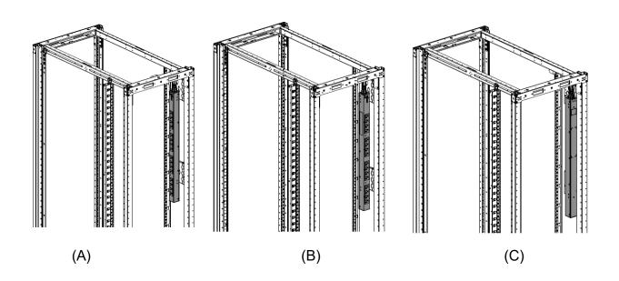
**NOTE:** The above installation methods are true for all vertical models except for the dual sided models. Those units can only mount on its side with outlets facing the back of the rack. Reference the dual sided PDU installation section for installation instructions.
