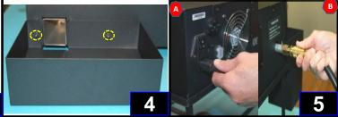
6-Pull cap on Air Regulator and turn to adjust air(A). Gage should read between 65-85 psi.Power unit ON. (B). 7-Connect hose to the outlet in front of the dispenser.
