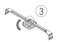
ROTATE BOX ASSEMBLY CLOCKWISE TO LOCK BOX INTO PLACE (LOCKING TABS ON BOX CLIP SHOULD ENGAGE SLOTS IN BAR HANGER)
