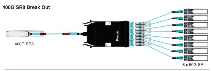
Figure 4: Review of 400Gb SR8: (1) x 400G SR8 to (4) of 2 x 50G SR Breakout Application (MPO24)
