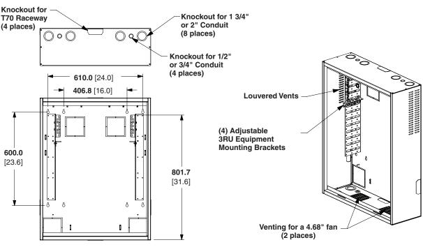
Dimensions are in metric. [Dimensions in brackets are inches].
