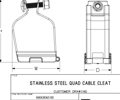
DATASET FILE NAME 00653ENZ-DC/00A THIRD ANGLE CUSTOMER PROJECTION MATERIAL RAWING NUMBER 316L STAINLESS STEEL 00653ENZ\_DC 00A 08/25/21 ACC ADAH ALP INITIAL RELEASE 104453 SIZE DRAWN BY DATE SCALE REV ΒY CHK DATE APR ECN DESCRIPTION DFTR 4/28/21 ADAH NONE SHEET 1 OF 1
