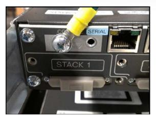
Figure 23: Ground cable connection to the Fiber switch.
