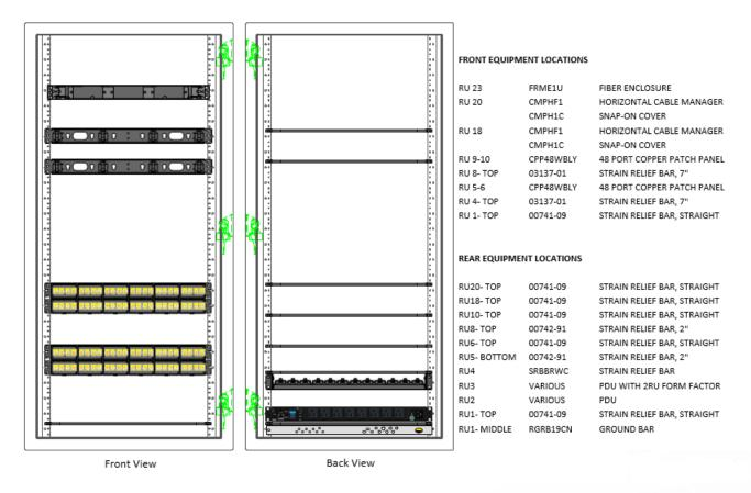
Figure 25: Industrial Distribution Frame (IDF) with Access Control Equipment Elevation
