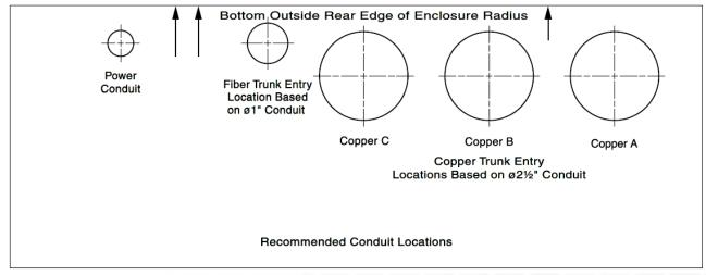
**Figure 6: Recommended Conduit Location Template**
