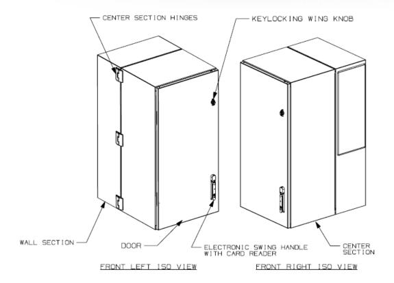
Figure 26: Isometric View Showing the Steel IDF Enclosure Construction
