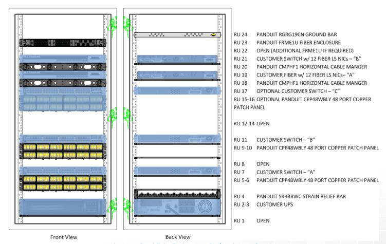
Figure 1: Industrial Distribution Frame (IDF) Equipment Elevation
