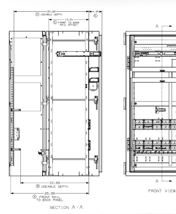
Figure 4: IDF Section showing the useable depth of the enclosure.
