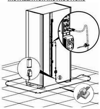
Connect the RJ-45 jack on the Rope Fluid Leak Sensor assembly to a sensor port on the iPDU or Sensor Hub (Panduit PN: EF001) and secure with provided Adhesive Backed Mounts and Cable Ties.
