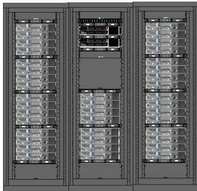
Example of 3 cabinet Pod with 40 2 RU servers distributed over 3 cabinets with 2 ToR switches in center cabinet requires 80 SFP+ cables with longest cable of 4m
