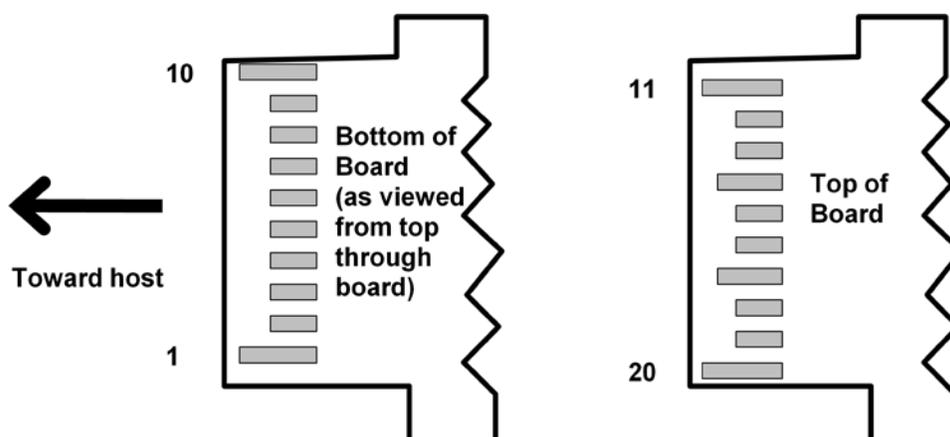
**SFP Connector Module Contact Assignments
