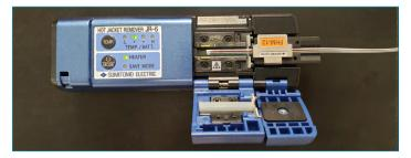
Figure 7: Removing the jacket from the fiber.
