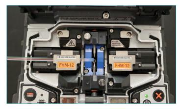
**Figure 10:** Inserting the bare fiber(s) into the Fusion Splicer. Sheath Clamp shown on the left.
