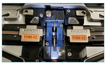
Figure 14: Image of completed arc process, fibers fused.
