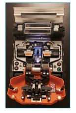
**Figure 4:** Fusion Splicer shown open, Fiber Sheaths closed.
