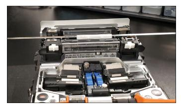
Figure 16: Spliced Fiber with splicing sleeve in place, being laid into Oven 1.
