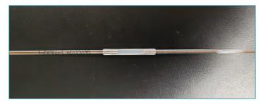
Figure 1: 12-ribbon fiber, post arc procedure.
