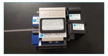
Figure 9: Cleaving the bare fiber(s).
