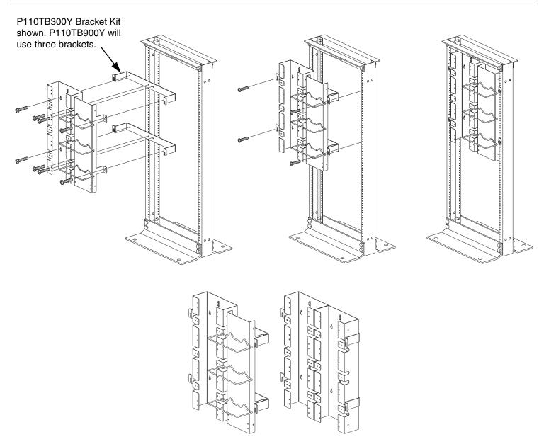
The brackets can be used to mount one tower and one vertical cable manager or two towers. The brackets will not accommodate two vertical cable managers. The vertical cable manager can be mounted only on the right side, as shown, using the labeled holes below.
