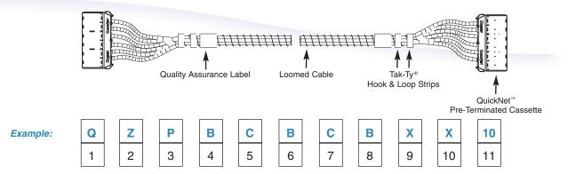
Example – The above part number is a 10 foot QuickNet<sup>™</sup> Cable Assembly constructed of Category 6A, UTP, plenum cable (blue) with a pre-terminated cassette (blue jacks installed) on each end.
