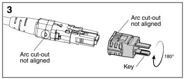
Rotate outer housing 180° so arc cut-out is on the opposite side.
