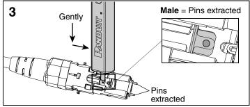
Insert tool into hole, press down gently, and push forward to advance connector pins to the male state. Repeat process in opposite direction to retract pins for female state. 2 CAUTION! Only Panduit tool is to be used for gender change. Use of any other tool can cause fiber damage and will void the product warranty. hole
