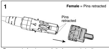
Remove outer housing per polarity changeover instructions.
