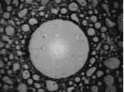
Oil/Liquid residue on MPO connector core and cladding
