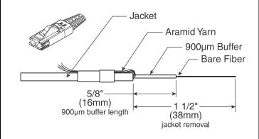
The plug side is not intended to be terminated using 900µm buffered fiber.
