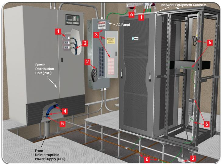
Power Distribution Units (PDUs) provide power to AC panels. AC panels provide power to network equipment cabinets.
