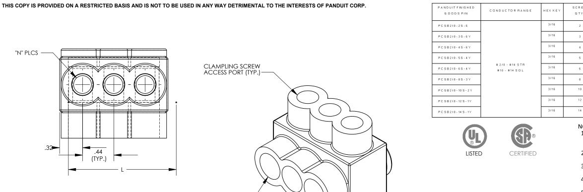
THREE PORT CONNECTOR BLOCK SHOWN WITH PLASTIC CLOSURE PLUGS REMOVED. SEE TABLE FOR DIMENSIONS OF PARTS WITH ADDITIONAL PORTS
