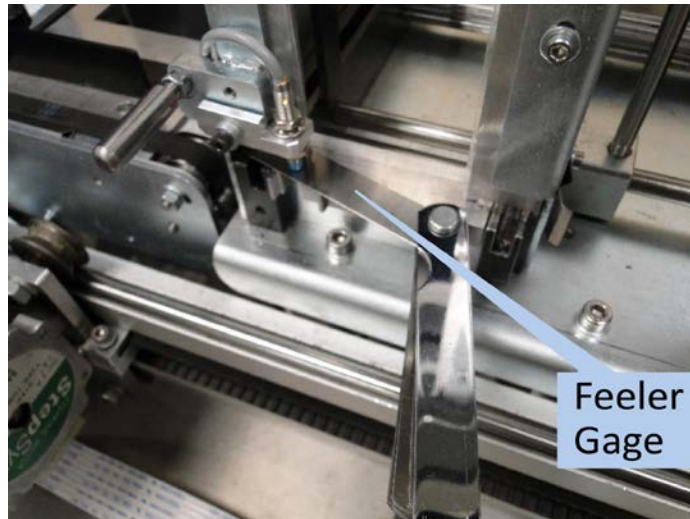
Figure 13 Feeler Gage placement under LH gate
