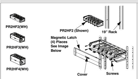
Install the managers to the rack with #12-24x1" screws provided. Install the cover to the manager by positioning the magnetic latches near the hinge pins of the manager.
