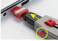
d) Remove device by pulling the key
