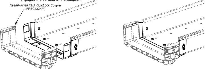
5. With the *FIBERRUNNER* 12x4 *QUIKLOCK* Coupler in place, a section of *FIBERRUNNER* 12x4 Channel and/or any *FIBERRUNNER* 12x4 Fitting can be installed to continue the fiber pathway.
