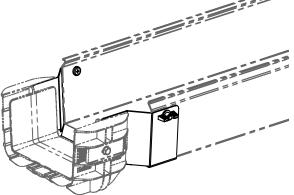
5. With the FIBERRUNNER 6x4 QUIKLOCK Coupler in place, a section of FIBERRUNNER 6x4 Channel and/or any FIBERRUNNER 6x4 fitting can be installed to continue the fiber pathway.
