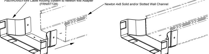
With the adapter held in place, mark all five (5) mounting hole locations of the adapter on to the channel 2. section. Remove the adapter and with a <sup>9</sup>/<sub>32</sub>" diameter drill bit create five (5) mounting holes in the channel. Please note that before the drilling operation begins, that all cables, etc. are out of the path of the drilling bit.
