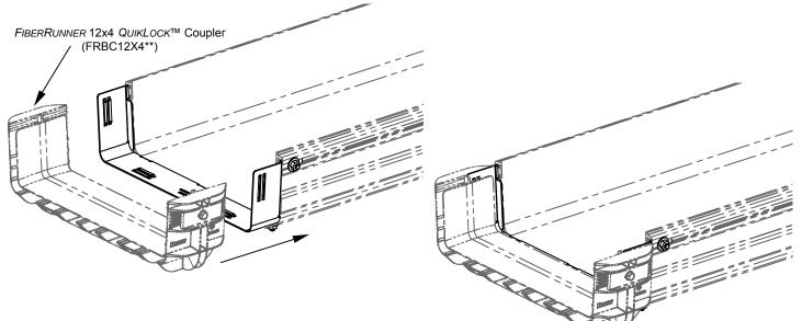
4. With the *FIBERRUNNER* 12x4 *QUIKLOCK* Coupler in place, a section of *FIBERRUNNER* 12x4 Channel and/or any *FIBERRUNNER* 12x4 fitting can be installed to continue the fiber pathway.
