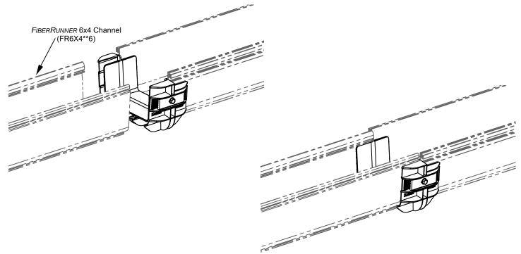
In the event that disassembly is required, connections made with the *FIBERRUNNER* 6x4 Cable Routing System to ADC 4x6 FiberGuide Adapter can be easily disconnected as follows:
