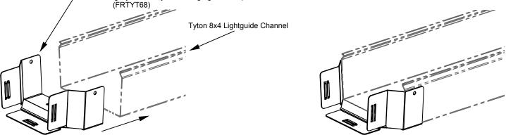
2. With the adapter held in place, mark all four (4) mounting hole locations of the adapter on to the channel section. Remove the adapter and with a <sup>9</sup>/<sub>32</sub> diameter drill bit create four (4) mounting holes in the channel. Please note that before the drilling operation begins, that all cables, etc. are out of the path of the drilling bit.
