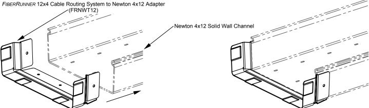
2. With the adapter held in place, mark all five (5) mounting hole locations of the adapter on to the channel section. Remove the adapter and with a <sup>9</sup>/<sub>32</sub> diameter drill bit create five (5) mounting holes in the channel. Please note that before the drilling operation begins, that all cables, etc. are out of the path of the drilling bit.
