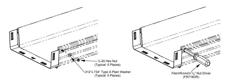
3. With the adapter secure to the ADC 4x12 FiberGuide Channel, align the extended ribs of the *FIBERRUNNER* 12x4 *QUIKLOCK* Coupler with the *FIBERRUNNER* Cable Routing System side of the adapter. Once aligned, push the adapter and the coupler together until the adapter is seated against the inner rib of the coupler. Please note that the slight amount of resistance that is felt is normal, indicating that the metal barbs of the coupler have engaged the surface of the adapter.
