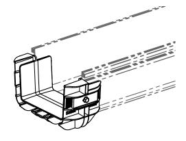
2. Next, align the *FIBERRUNNER* 6x4 Channel and/or fitting with the extended ribs of the *FIBERRUNNER* Cable Routing System side of the adapter. Once aligned, push the adapter and channel/fitting together until the channel/fitting is seated against the inner rib of the adapter.
