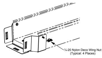
4. With the adapter secure to the Tyton 8x4 Lightguide Channel, align the extended ribs of the FIBERRUNNER 6x4 QUIKLOCK<sup>™</sup> Coupler with the FIBERRUNNER Cable Routing System side of the adapter. Once aligned, push the adapter and the coupler together until the adapter is seated against the inner rib of the coupler. Please note that the slight amount of resistance that is felt is normal, indicating that the metal barbs of the coupler have engaged the surface of the adapter.
