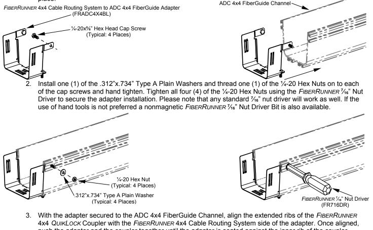
3. With the adapter secured to the ADC 4x4 FiberGuide Channel, align the extended ribs of the FIBERRUNNER 4x4 QUIKLOCK Coupler with the FIBERRUNNER 4x4 Cable Routing System side of the adapter. Once aligned, push the adapter and the coupler together until the adapter is seated against the inner rib of the coupler. Please note that the slight amount of resistance that is felt is normal, indicating that the metal barbs of the coupler have engaged the surface of the adapter.
