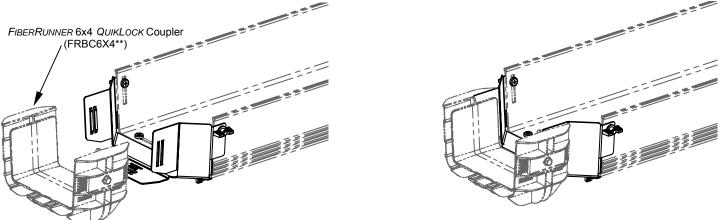
5. With the FIBERRUNNER 6x4 QUIKLOCK Coupler in place a section of FIBERRUNNER 6x4 Channel and/or any FIBERRUNNER 6x4 fitting can be installed to continue the fiber pathway.
