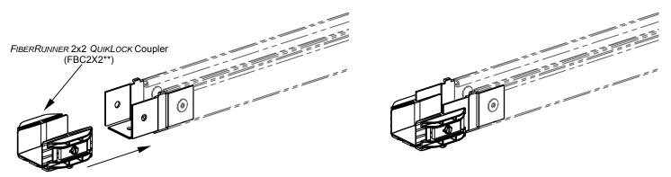
5. With the *FIBERRUNNER* 2x2 *QUIKLOCK* Coupler in place, a section of *FIBERRUNNER* 2x2 Hinged or Hinged Slotted Channel and/or *FIBERRUNNER* 2x2 fitting can be installed to continue the fiber pathway.
