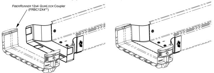
5. With the *FIBERRUNNER* 12x4 *QUIKLOCK* Coupler in place, a section of *FIBERRUNNER* 12x4 Channel and/or any *FIBERRUNNER* 12x4 Fitting can be installed to continue the fiber pathway.
