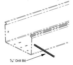
3. Reattach the adapter and realign all five (5) of the mounting holes. With the adapter held in place, insert one (1) of the ¼-20x<sup>5</sup>/<sub>6</sub>" Nylon Phillips Binder Head Screws through each of the mounting holes from the inside of the channel. Be sure that all five (5) of the binder head screws are pointing outward away from the adapter. Thread one (1) of the ¼-20 Nylon Deco Wing Nuts on to each of the binder head screws and hand tighten.
