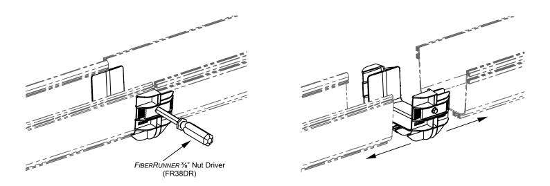
2. The bolts of the adapter can then be re-tightened. Please be aware not to over tighten the bolts. Once tightened, the *FIBERRUNNER* 6x4 Cable Routing System to ADC 4x6 FiberGuide Adapter is ready for use once again.
