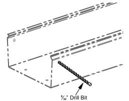
3. Reattach the adapter and realign all four (4) of the mounting holes. With the adapter held in place, insert one (1) of the ¼-20x% Nylon Phillips Binder Head Screws through each of the mounting holes from the inside of the channel. Be sure that all four (4) of the cap screws are pointing outward away from the adapter. Thread one (1) of the ¼-20 Nylon Deco Wing Nuts on to each of the binder head screws and hand tighten.
