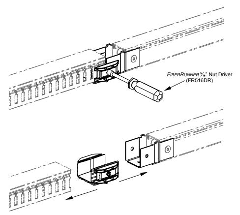
2. The bolts of the coupler can then be re-tightened. Please be aware not to over tighten the bolts. Once tightened, the *FIBERRUNNER* 2x2 *QUIKLOCK* Coupler is ready for use once again.
