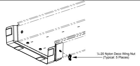
4. With the adapter secure to the Newton 4x12 Solid Wall Channel, align the extended ribs of the FIBERRUNNER 12x4 QUIKLOCK<sup>™</sup> with the FIBERRUNNER Cable Routing System side of the adapter. Once aligned, push the adapter and the coupler together until the adapter is seated against the inner rib of the coupler. Please note that the slight amount of resistance that is felt is normal, indicating that the metal barbs of the coupler have engaged the surface of the adapter.
