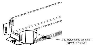
4. With the adapter secure to the Warren & Brown 8x4 Lightpath Channel, align the extended ribs of the FIBERRUNNER 6x4 QUIKLOCK<sup>™</sup> Coupler with FIBERRUNNER Cable Routing System side of the adapter. Once aligned, push the adapter and the coupler together until the adapter is seated against the inner rib of the coupler. Please note that the slight amount of resistance that is felt is normal, indicating that the metal barbs of the coupler have engaged the surface of the adapter.
