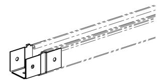
2. With the coupler held in place against the other channel section, mark all three (3) mounting hole locations of the coupler on to the channel section. Remove the coupler and with a <sup>5</sup>/<sub>6</sub>" diameter drill bit create three (3) mounting holes in the other channel. Please note that before the drilling operation begins, that all cables, etc. are out of the path of the drilling bit.
