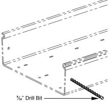
3. Reattach the adapter and realign all five (5) of the mounting holes. With the adapter held in place, insert one (1) of the ¼-20x%" Nylon Phillips Binder Head Screws through each of the mounting holes from the inside of the channel. Be sure that all five (5) of the binder head screws are pointing outward away from the adapter. Thread one (1) of the ¼-20 Nylon Deco Wing Nuts on to each of the binder head screws and hand tighten.
