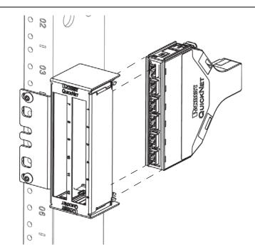
The QuickNet Zero RU Bracket can also be mounted directly to the cabinet rail with the screws provided.
