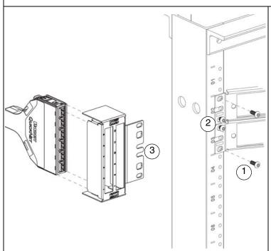
The QuickNet Zero RU Bracket can be mounted onto a previously installed equipment bracket using existing screws:
