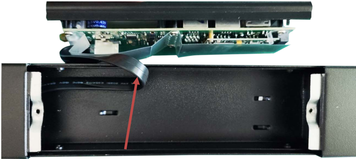
Figure 79: RJ45 Cable for the Network Controller
