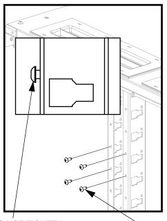
**DO NOT TIGHTEN** (Leave Gap Between Screw and Cabinet Post)
