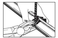
3. Use pliers utilizing tension steps on tie to tighten completely.
