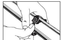
2. Position cable against tie spacer and thread tail through slot in head. Push upwards on body of tie until snug.
