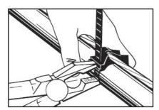
3. Use pliers utilizing tension steps on tie to tighten completely.
