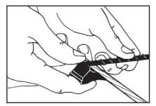
1. Snap groove portion of tie onto support strand.
