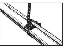
4. Support tie shown when properly installed. If releasability is not required, tip can be cut off.
