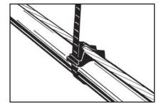
4. Support tie shown when properly installed. If releasability is not required, tip can be cut off.
